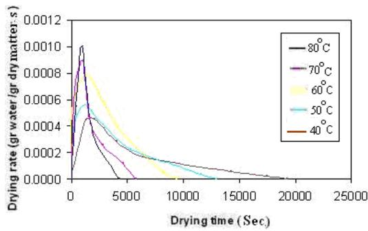
**Fig 5.** Drying rate changes with drying time for 2mm thickness
