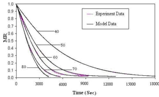
**Fig 2.** Effect of drying air temperature on drying time for 2mm thickness
