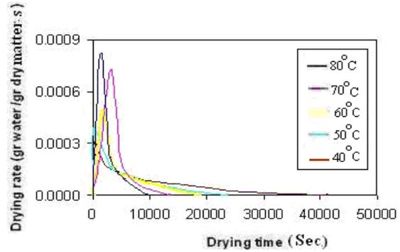
**Fig 6.** Drying rate changes with drying time for 4mm thickness
