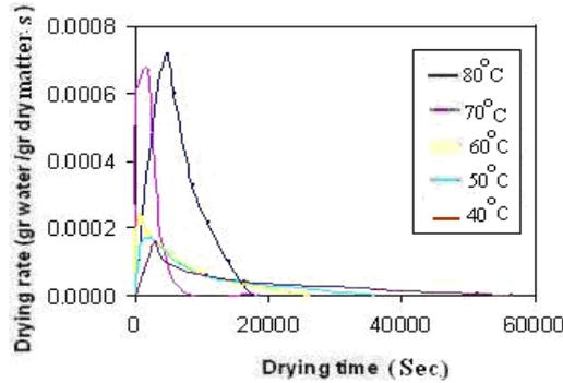
**Fig 7.** Drying rate changes with drying time for 6mm thickness
