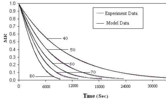
**Fig 3.** Effect of drying air temperature on drying time for 4mm thickness
