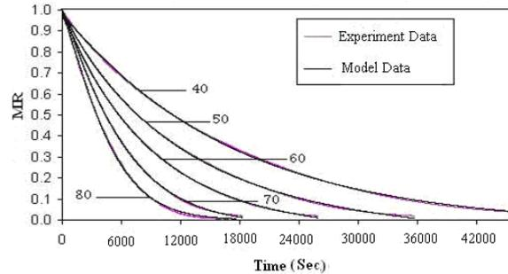
**Fig 4.** Effect of drying air temperature on drying time for 6mm thickness
