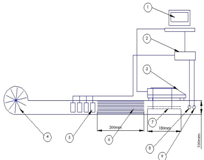
**Fig 1.** Schematic diagram of the drying system for measurement of the thin-layer parameters of apple slices. 1. PC; 2. microcontroller; 3. digital balance; 4. fan; 5. heating elements; 6. duct and tunnel; 7. trays; 8. temperature sensor; 9. relative humidity sensor.
